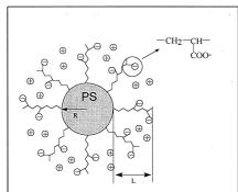
Fig. 1: Sketch of the spherical polyelectrolyte brushes investigated here: Linear chains of poly(acrylic acid) (PAA) are chemically grafted onto the surface of a colloidal poly(styrene) particle <sup>14-15</sup>.
