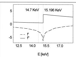
Fig. 2: The parameters f' and f'' calculated for Rubidium using the routine of Chantler<sup>24</sup>. The perpendicular lines indicate the energies for which the model calculations have been done.
