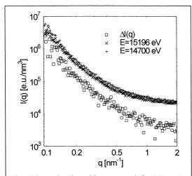
Fig. 4: Scattering intensities measured far below the adsorption edge (+++) and in the immediate vicinity (xxx). The squares mark the difference between the two scattering intensities according to eq.(8). (see text for further explanation).
